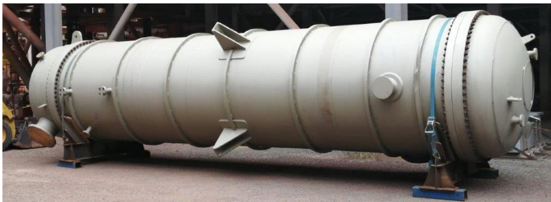
Figure 2. HEX unit tubed with Superhex.
